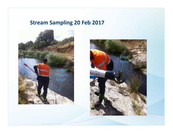
In response to Action 301116\_2 *Cleanaway to report on whether the high salinity reading at MPCL04 was when there was no flow in the creek*, a flow meter is being used in the creek which will provide more data. Salinity levels are tested every 5m along the stream for 500m in either direction from the landfill.
